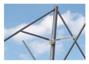
The FMP antennas are easy to install and are pre tuned at the factory. The diagram below depicts a two bay antenna (FMP-2). The antennas will produce the best radiation pattern if mounted to a small support pole, and installed with free space above and below the antenna. The numbers provided are for operation at 98 MHz.
